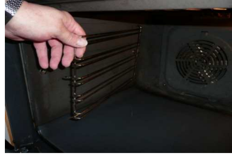
Risten i siden udtages for rengøring. Remove the side grates before cleaning.
